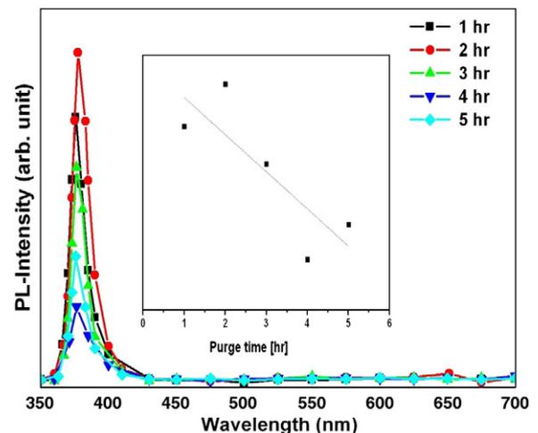
**Fig. 5.** Change of PL intensity of ZnO thin film by annealing in vacuum at 300 °C according to the vacuum treatment time.
