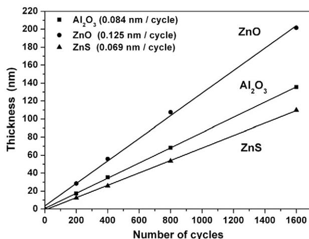
Fig. 1. Film thickness of Al<sub>2</sub>O<sub>3</sub>, ZnO and ZnS on Si(100) as a function of the number of cycles.
