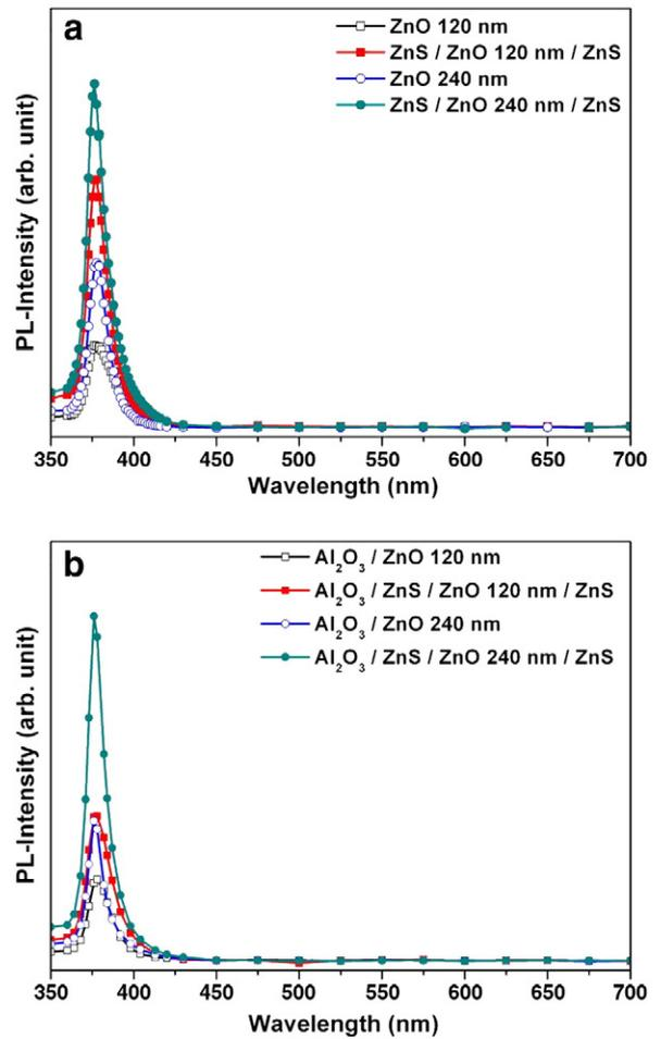
**Fig. 4.** Photoluminescence spectra of the ZnO single layer and ZnS/ZnO/ZnS multi-layer according to the ZnO thickness (120 nm and 240 nm) on (a) Si(100) and (b) Si/Al<sub>2</sub>O<sub>3</sub>.
