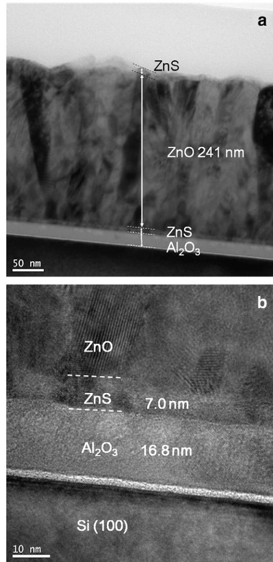
**Fig. 3.** Cross-sectional transmission electron microscopy images of Si/Al<sub>2</sub>O<sub>3</sub>/ZnS/ZnO/ZnS multi-layers: (a) entire range (×100,000) and (b) high-resolution (×300,000) image of the interface between the ZnO and Si wafer.
