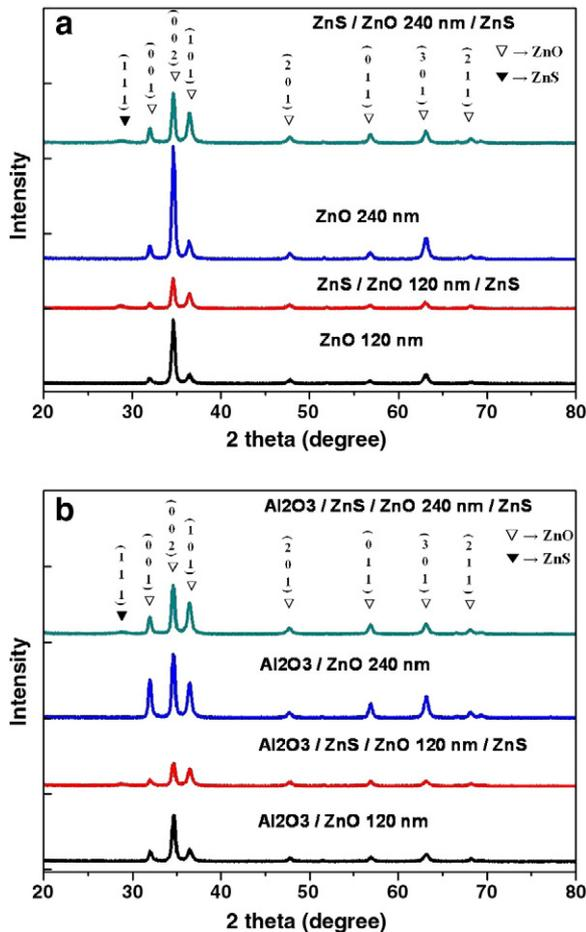
**Fig. 2.** X-ray diffraction patterns of the ZnO single layer and ZnS/ZnO/ZnS multi-layer according to the ZnO thickness (120 nm and 240 nm) on (a) Si(100) and (b) Si/Al<sub>2</sub>O<sub>3</sub>.
