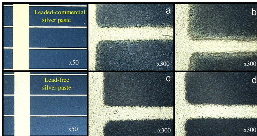
Fig. 4. Optical microscope images of fired silver front pastes corresponding to (a) Ferro CN-33-462 (peak fired temperature,  $T_{peak}$ : 750 °C), (b) Ferro CN-33-462 ( $T_{peak}$ : 910 °C), (c) FS01 ( $T_{peak}$ : 750 °C) and (d) FS01 ( $T_{peak}$ : 910 °C) pastes.
