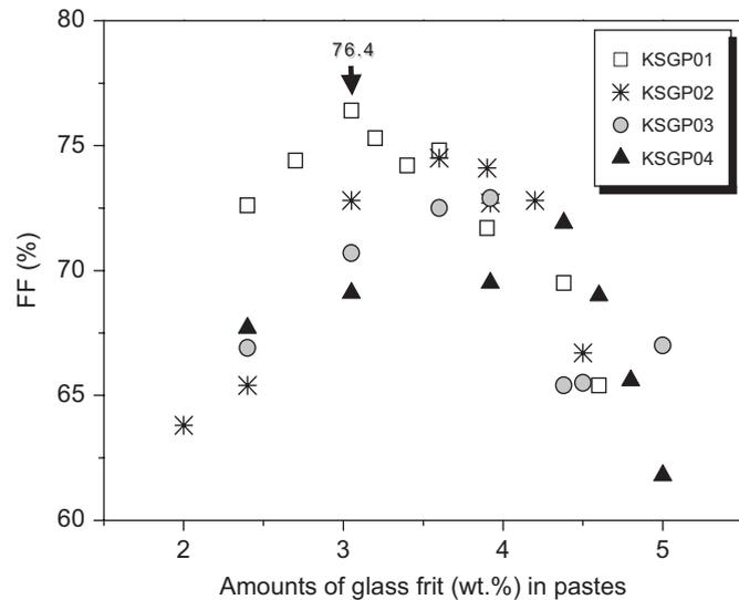
Fig. 3. Influence of glass frits with a different mean particle size as a function of their contents in pastes on the FF of solar cells.
