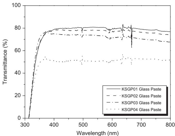
**Fig. 2.** Transmittance patterns of the different glass pastes after being fired at 600 °C for 30 min.
