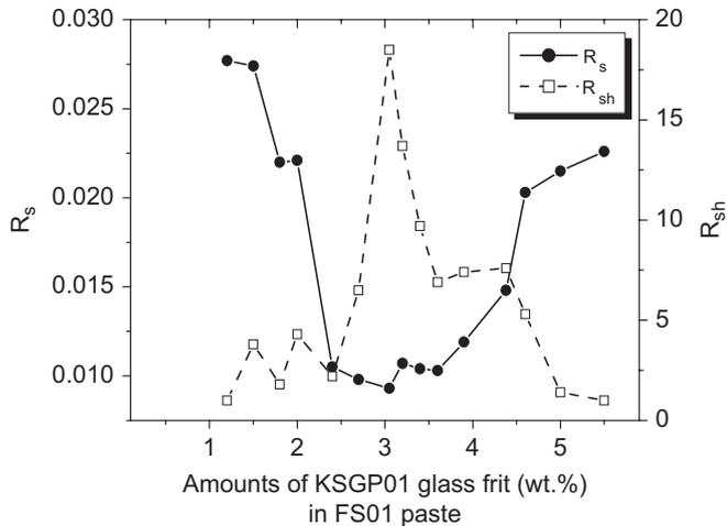
**Fig. 5.** The change of the series resistance ( $R_s$ ) and shunt resistance ( $R_{sh}$ ) as a function of amounts of KSGP01 glass frit (wt%) in FS01 pastes.
