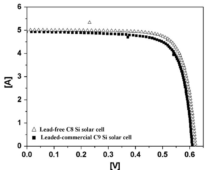
Fig. 8. Current–voltage ( $I$ – $V$ ) curves of the C8 and C9 Si solar cells fabricated with lead-free silver paste (FS08) and leaded commercial silver paste (CN33-462) on emitters having a sheet resistance of  $45\ \Omega/\text{sq}$ .
