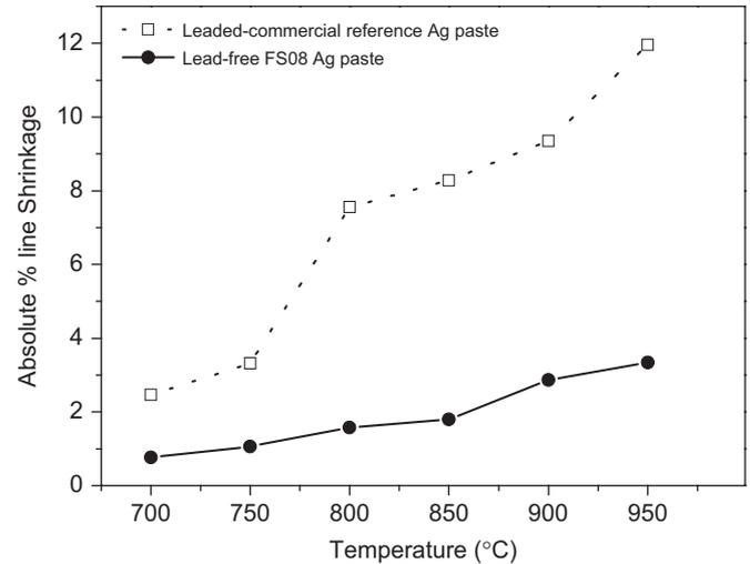
**Fig. 6.** The dependence of shrinkage in fired line patterns as a function of firing temperature.
