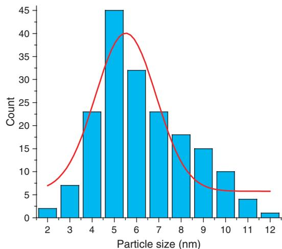
**Fig. 3.** Transmission electron micrograph image and particle size distribution histogram of dodecylamine stabilized silver nanoparticles. Insert: HRTEM image of silver nanoparticles.
