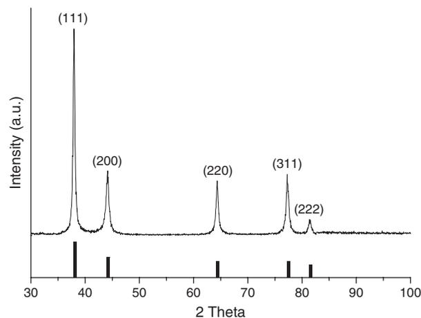
Fig. 1. XRD pattern of dodecylamine capped silver nanoparticles (bar: JCPDS no. 04-0783).
