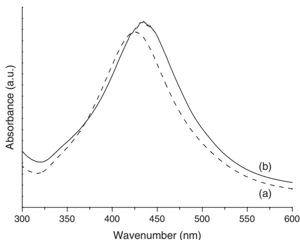
**Fig. 2.** UV-vis absorption spectrum of (a) dodecylamine capped on silver nanoparticles (b) silver nanoparticles (0.5 wt%) included in polycarbonate films.
