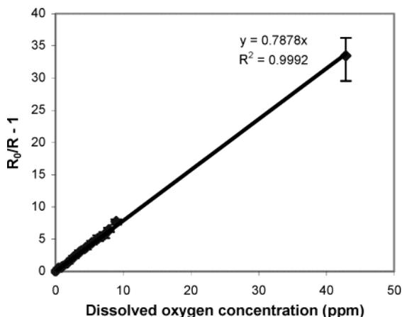
Figure 3. Stern–Volmer plot of relative fluorescence intensity ratios for ratiometric ormosil PtOEPK PEBBLES.  $R_0$  is the ratio between the fluorescent intensities of PtOEPK and OEP in the absence of oxygen, and  $R$  is the ratio at a given oxygen concentration.
