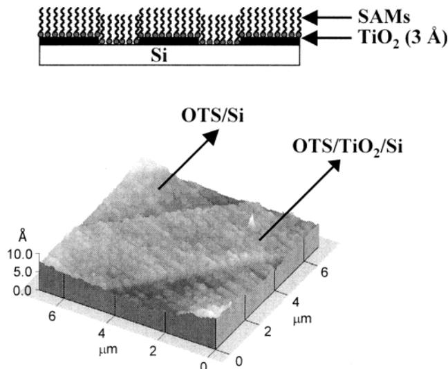
**Figure 8.** Scheme and AFM image of the OTS-based monolayer on the patterned TiO<sub>2</sub> thin film.
