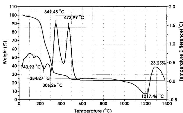
**Fig. 3.** TG/DTA analysis for  $\text{LiNbO}(\text{O}-2,6\text{-PhMe}_2)_4 \cdot 3\text{THF}$  (1) from room temperature to 1400°C, measured at 10°C/min in air atmosphere with a flow rate of 60.0 ml/min.
