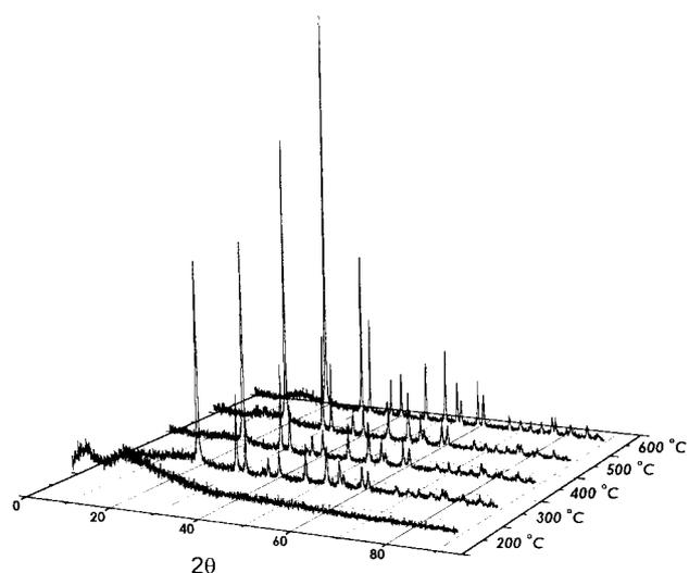
**Fig. 4.** XRD spectra for the low-temperature calcined precursors for 3 h (200–600°C).
