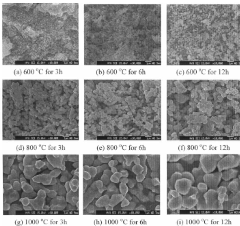
**Fig. 5.** SEM micrographs of the calcined  $\text{LiNbO}_3$  powders at 600 °C (a) for 3 h, (b) 6 h, (c) 12 h; at 800 °C (d) for 3 h, (e) 6 h, (f) 12 h; at 1000 °C (g) for 3 h, (h) 6 h, and (i) 12 h. Bar lengths represent 1  $\mu\text{m}$ .
