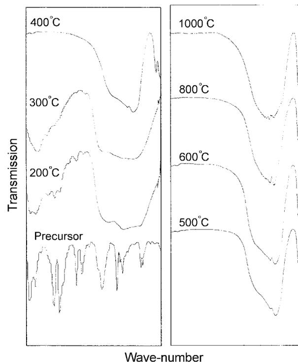
**Fig. 2.** FT-IR spectra for  $\text{LiNbO(O-2,6-PhMe}_2)_4 \cdot 3\text{THF}$  (**1**) and the calcined precursors ( $200\text{--}1000^\circ\text{C}$ ).
